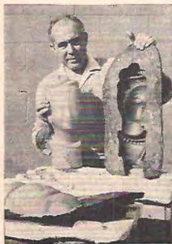
The ground glass will set in approximately thirty minutes at a temperature of 75 degrees. It can then be removed carefully from the mold.
